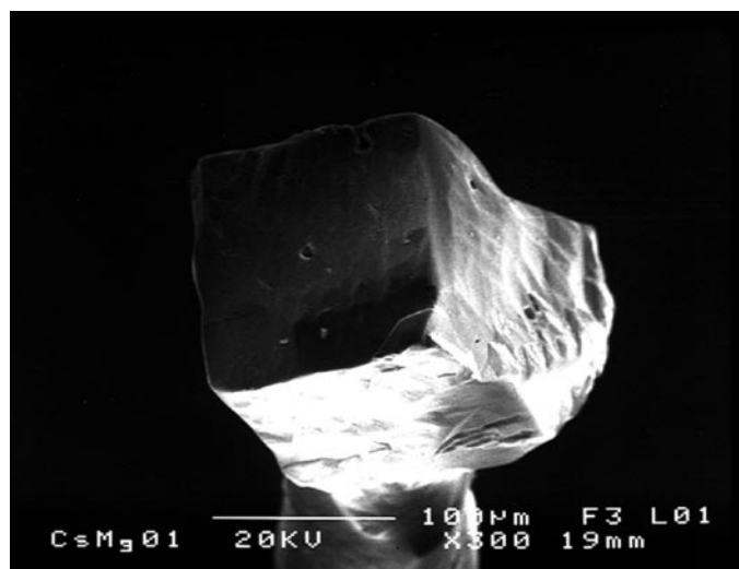
FIG. 2. SEM micrograph of the single crystal of \text{Cs}_3\text{Mg}_2\text{P}_6\text{O}_{17}\text{N} used in this study.
